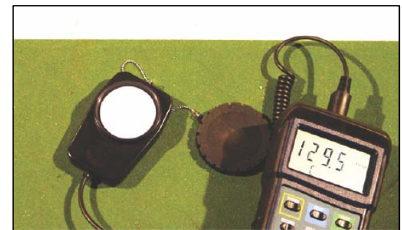
Reading at the Base Line: 129.5 foot candles
